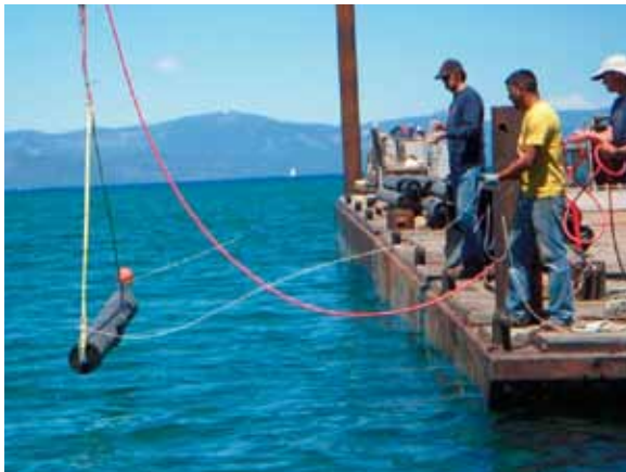
Release mechanism on barge helps researchers to lower barriers into water
