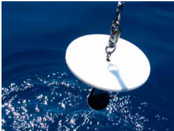
The Secchi disk has been used to measure clarity at Lake Tahoe since 1968 with measurements taken every 10-14 days
