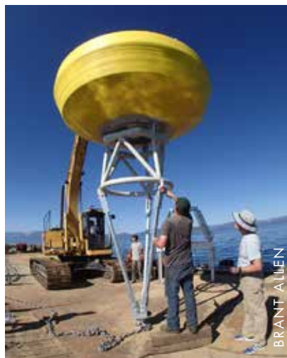
NASA-JPL BUOYS being assembled prior to deployment on Lake Tahoe
