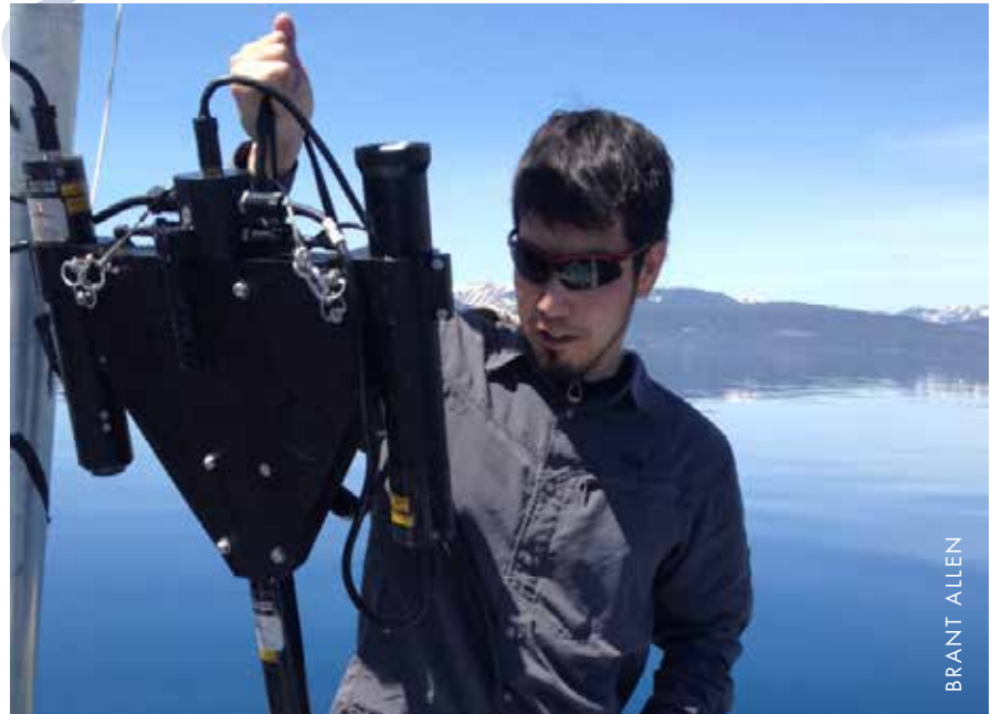
SHOHEI WATANABE takes radiometric profiles regularly to calibrate the buoy sensors
