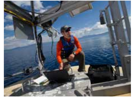
SHOHEI WATANABE on the NASA buoy uses hyperspectral radiometric measurements to measure the color of the lake
