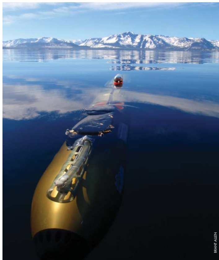
Autonomous underwater vehicle (AUV), known as Gavia, resembles a torpedo but is equipped with a broad suite of scientific instruments
