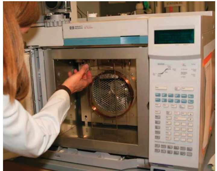
Anne Liston utilizes the gas chromatograph to measure fatty acids and study the transfer of nutrients through the food web
