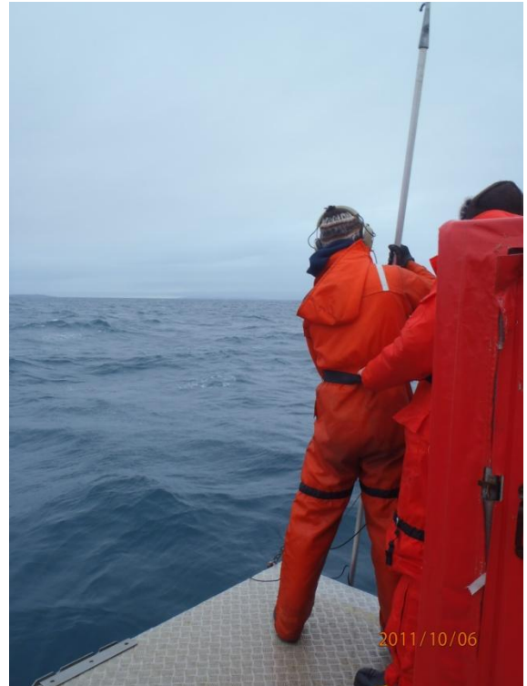
Andrew Hamilton working with the hydrophone to locate the AUV. Photo courtesy of Anna Crawford.
