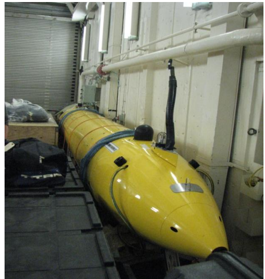
The AUV on board CCGS Louis S St-Laurent. Photo courtesy of Anna Crawford.
